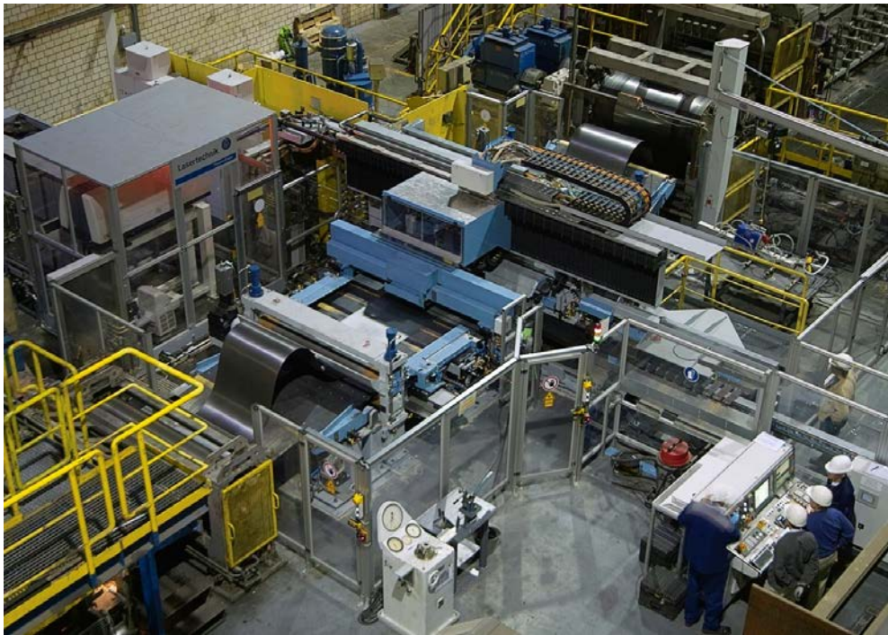
Figure 2: The WISCO Laser Welding Machine at ThyssenKrupp. The laser source, a 5 kW CO 2 laser, is mounted in a acrylic glass cage at the side of the line. Because of work safety (laser radiation, automatically moving machines) the entire laser welding machine is enclosed by an acrylic fence (optically thin for optical wavelength, optically thick for CO 2 laser radiation).
