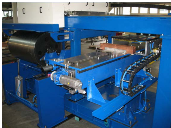
Figure 1: Tailored Blanks Production systems: Conti Laser Welding Machine (left); Laser Scratching System (right)
