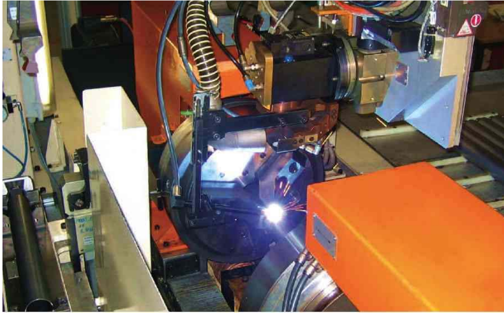
Fig. 8 Orbital welding system by ThyssenKrupp Lasertechnik: material flow from left (tube and base not welded) to the middle (welding station) to right (finished material).
