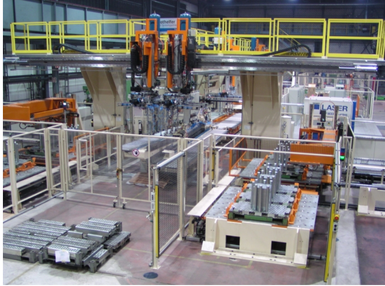
Fig. 1 Fully automatic laser welding line with continuous material feed.
