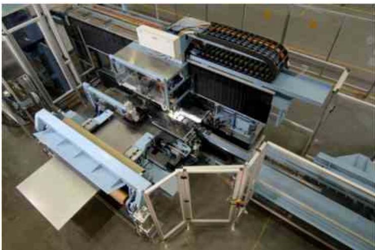
Fig. 5 Laser coil welding device with integrated laser edge cutting and seam marking.
