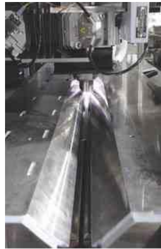
Fig. 5 Laser coil welding device with integrated laser edge cutting and seam marking.
