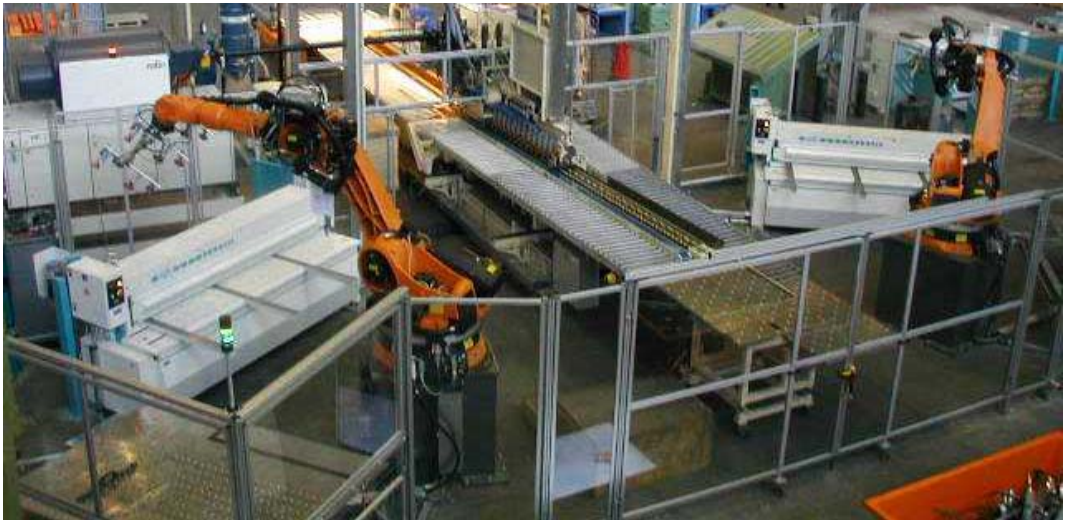
Fig. 4 Precision shears and 6-axis robots at the entry of a continuous laser welding line.
