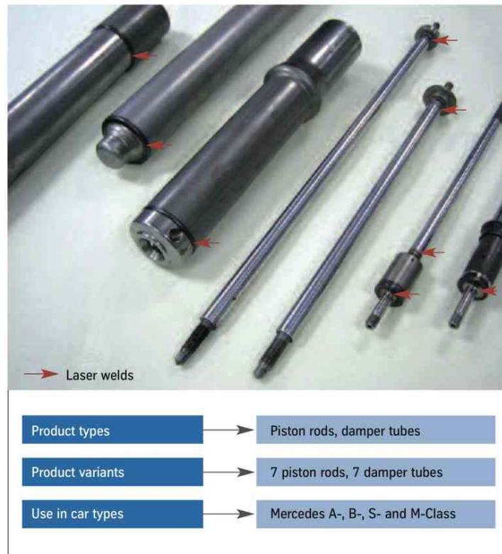
Fig. 7 Typical examples of Tailored Orbitals for shock absorber components (Mercedes-Benz).
