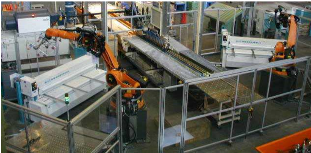
Figure 7. Precision shears and 6-axis robots at the entry of a laser welding line.
