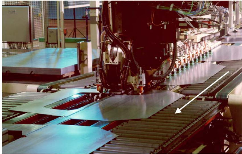
Figure 2: Fixed-optics welding machine with continuous material feed (arrow = feed direction).
