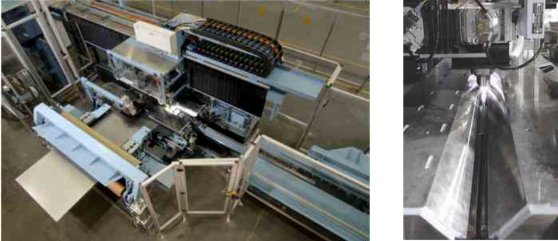
Figure 8: Laser coil welding device with integrated laser edge cutting and seam marking.
