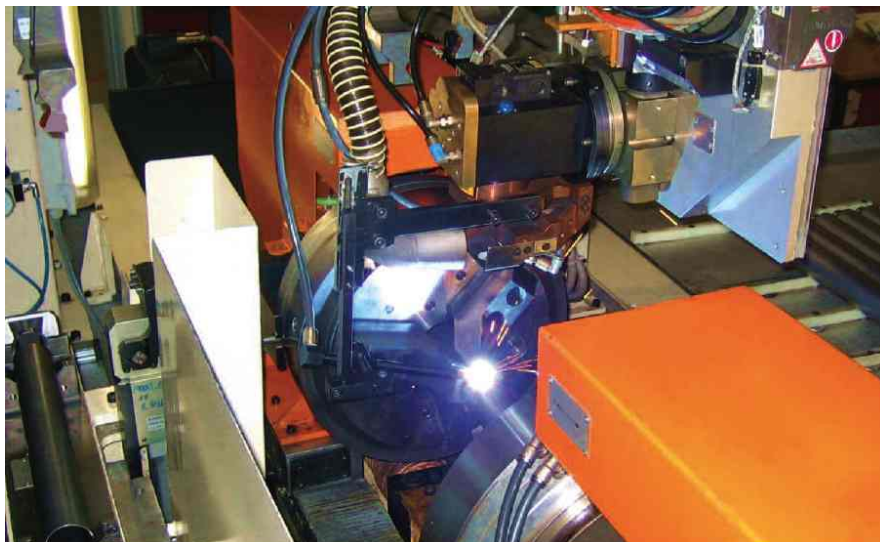
Figure 11: Orbital welding system by WISCO Lasertechnik: material flow from left (tube and base not welded) to the middle (welding station) to right (finished material).
