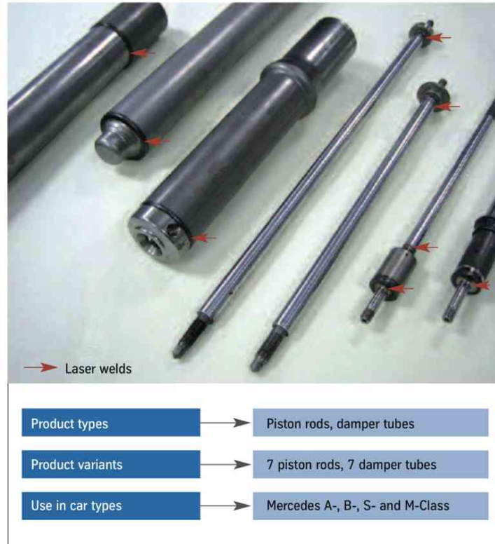
Figure 10: Typical examples of Tailored Orbitals for shock absorber components (Mercedes-Benz).
