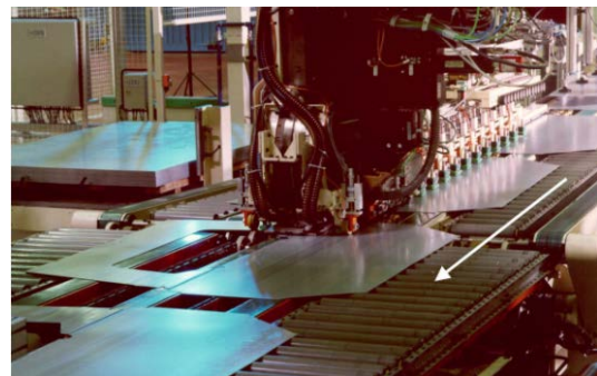
Fig.1 Fixed-optics welding machine with continuous material feed (arrow = feed direction)
